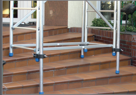
Stair support Cat. No. 410.10. Used to set up Scaffolding on the ground with different levels (RA 330). Possibility adjustable up to 600 mm.
