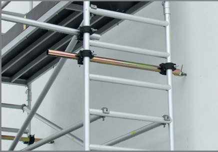
Anchor unit Cat. No. 220.09 (1.27 m) - for RA 1100, RA 1100S. Cat. No. 310.08 (1,77 m) - to RA 1100. It is used to fix scaffolding to the wall.
