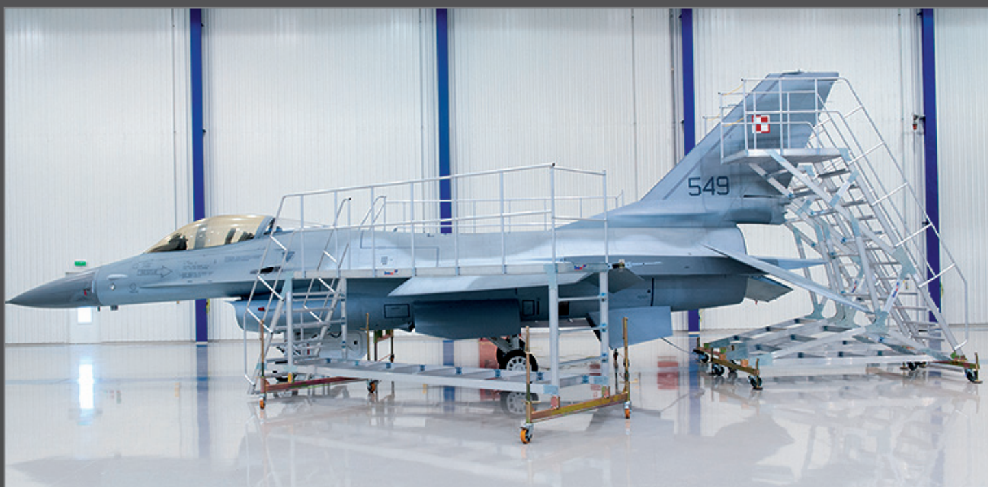
Specialized mobile scaffold sets with working platforms.
